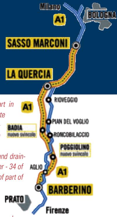
*Since 2006, Cipa has taken part in the construction of the "Variante di Valico," in order to strengthen the A1 motorway between Sasso Marconi and Barberino, where we have built structural and drainage shafts in considerable number - 34 of them - as well as the final lining of part of the main tunnel.*
